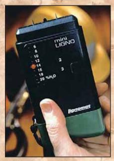
Moisture Meter - The MiniLigno-E is the most popular moisture meter on the market. Perfect for checking the MC of veneer, as well as lumber, fiberboard and other materials.
