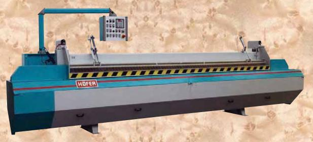
Standard Equipment 180mm saw blade 4 x 1.2 x 2" Milling cutter Pneumatic saw blade adjustment Automatic cutting tool feed Rear support table
