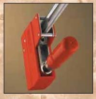
Bessey- K Body Clamps Superior strength, heavy duty components. Sustains clamping pressure throughout pad surface. Durable plastic clamping pads, spindle, steel rail, and internal parts are all replaceable. Clamping area of 3 1/2" x 1 3/4". Clamping pressure of up to 1000 lbs.
