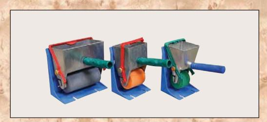
**Pizzi** Glue Dispenser - PVA glue is stored in the tank under pressure. The operator squeezes the handle to allow the flow of glue. Glue is released through the nozzle on demand, providing an even, consistent and continuous adhesive coating to the workpiece. Easy cleanup of nozzles with faucet adapter.
